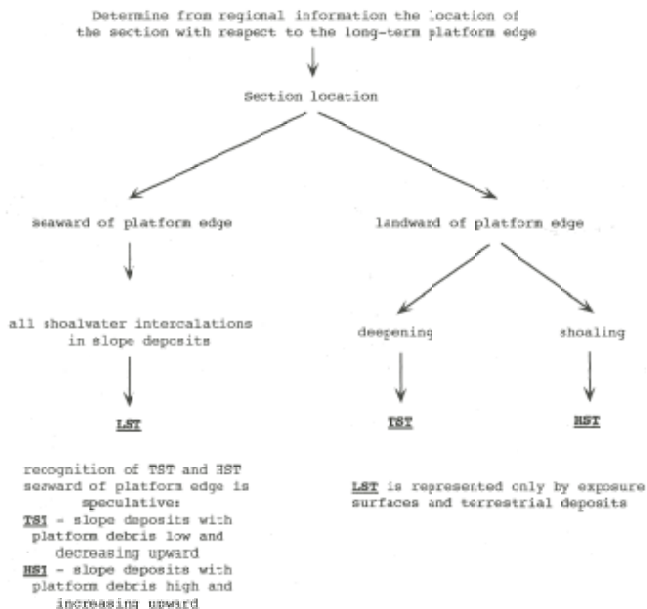
Fig.5-12 Identification of system tracts in a single section or borehole. This technique is more speculative than cross-section approach, relying on proxy indicators such as deepening and shoaling trends. The position of the section with respect to the long-term margin is required as input.
