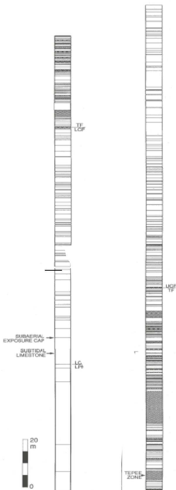
Fig. 5-18 Sequence stratigraphy of gradual change, demonstrated on a Triassic section on the Latemar atoll of the Southern Alps of Italy. Columns show over 200 m of platform deposits; sedimentation is distinctly cyclic throughout. Darker shades indicate more supratidal deposits, blank intervals are purely subtidal. LPF- largely subtidal cycles; LCF - lower subtidal-supratidal cycles; TF - tepee cycles, dominated by supratidal deposits; UCF - upper subtidal-supratidal cycles. Despite the absence of obvious breaks in the record, shoaling and deepening trends permit subdivision into sequences and systems tracts as indicated in Fig. 5-19. After Goldhammer et al. 1990.
