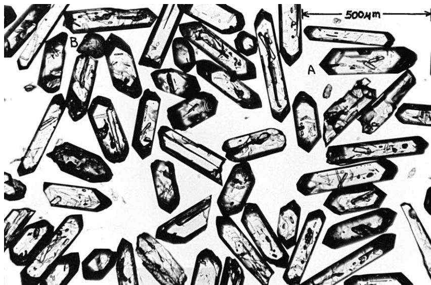
Fig. 9. A typical population of FCT zircons at 90\times magnification. Zircon B is a well-rounded “pink” Precambrian zircon. Zircon A is further magnified in Fig. 10.
